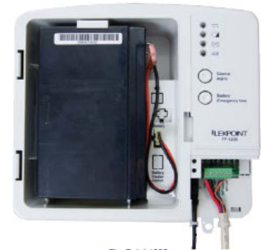
FlexPoint 1230 Shown with cover removed, battery, auxiliary power cable and NID hook-up cable
